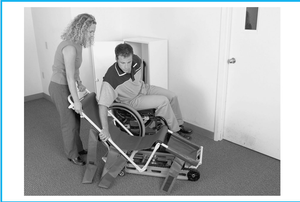
Exhibit 7.67 Person transferring from wheelchair to stair descent device. (Photo courtesy of Garaventa Lift)
