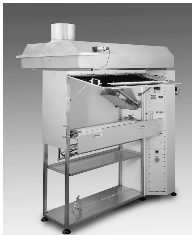
Exhibit S3.11 Flooring radiant panel tester apparatus. (Courtesy of Fire Testing Technology Ltd.)
