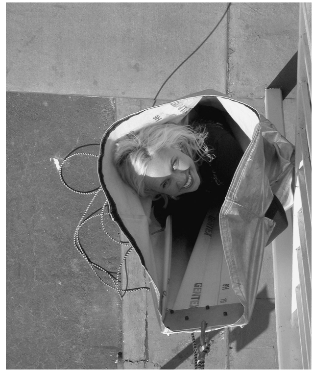
Exhibit C.2 Evacuee inside protective suit while using controlled descent device. (Photo courtesy of High-Rise Escape Systems, Inc.)
