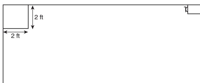
FIGURE A.8.7.5.1.6 Permitted Obstruction on Wall Opposite Sidewall Sprinkler.
