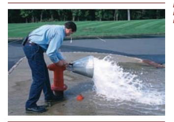
**EXHIBIT III.1** A Flow Diffuser in Use During a Hydrant Flow Test.
