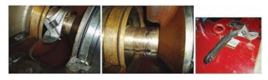
**EXHIBIT II.4.9** Fire Pump Damage from Careless Installation and Maintenance Procedures. (Courtesy of Aon Fire Protection Engineering)
