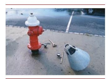
**EXHIBIT III.3** Diffuser – Slot for Pitot Tube Insertion.
