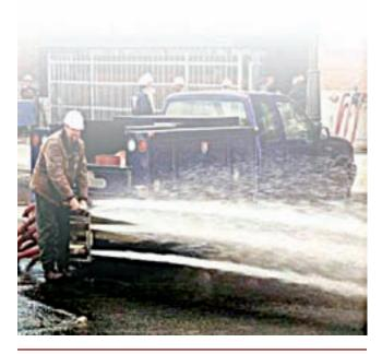
**EXHIBIT II.14.8** Determining Flow Using a Pitot Gauge. (Courtesy of Underwood Fire Equipment, Inc.)
