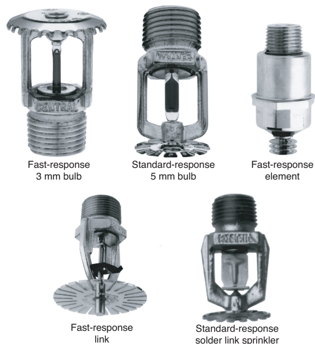
FIGURE A.5.3.1.1 Sprinkler Operating Element Identification.
