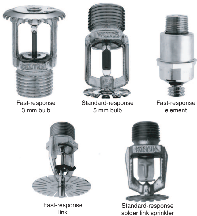
FIGURE A.5.3.1.1 Sprinkler Operating Element Identification.
