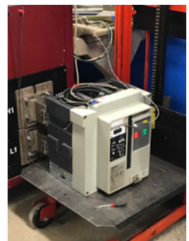
Primary Injection Testing
