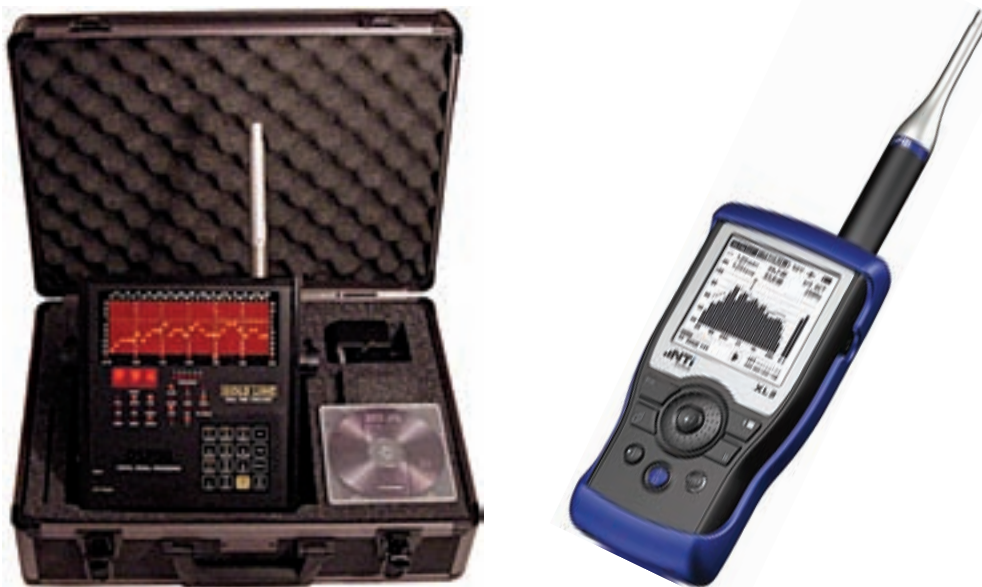
Combination Sound Pressure Level Meter/Analyzer and Speech Intelligibility Meter (left) and XL2 Audio and Acoustic Analyzer Displaying Basic STI-PA Result (right). [Sources: (left) Gold Line, West Redding, CT; (right) NTI Americas, Tigard, OR]
