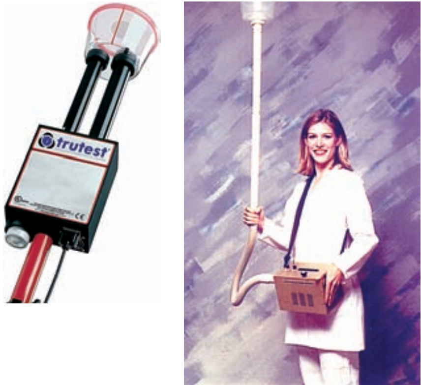
Test Equipment. (Left) Smoke Detector Sensitivity Tester (Courtesy of SDi, LLC, Neptune, NJ); (Right) Technician Using Calibrated Test Instrument. (Source: Gemini Scientific, Sunnyvale, CA)
