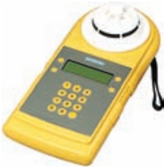
Device Programming Unit and Smoke Detector. (Source: Siemens Building Technologies, Fire Safety Division, Florham Park, NJ)
