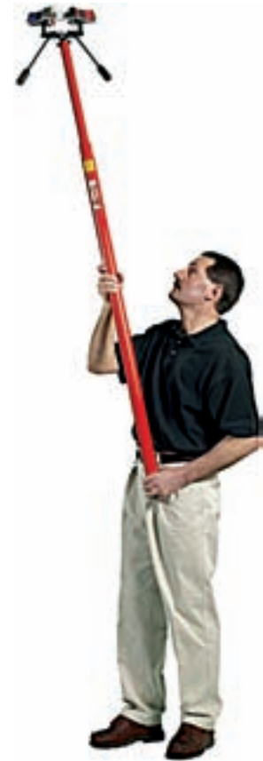
Removal Tool Used to Remove Detectors on High Ceilings. (Courtesy of SDi, LLC, Neptune, NJ)
