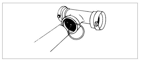
Fig. 27. Glass fiber-reinforced composite pipe, cast iron fitting and transition gasket.
