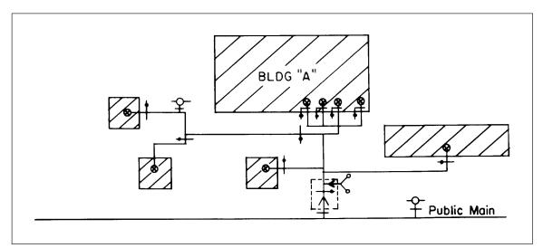
Fig. 32. System with manifolded riser arrangement.
