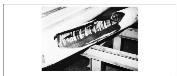
Fig. 41. High pressure hydro break.
