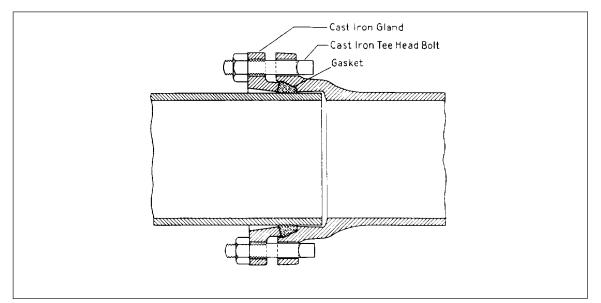
Fig. 19. Standardized mechanical joint.
