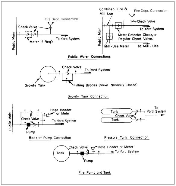
Fig. 28. Connections from water supplies.
