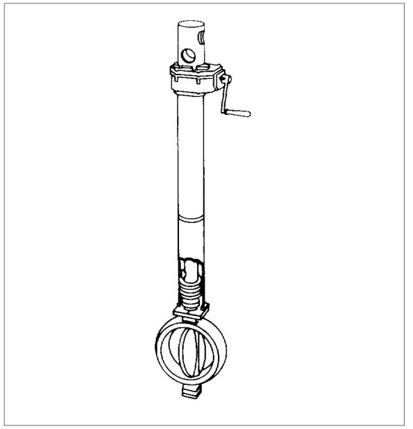
Fig. 11. Post indicator valve assembly.
