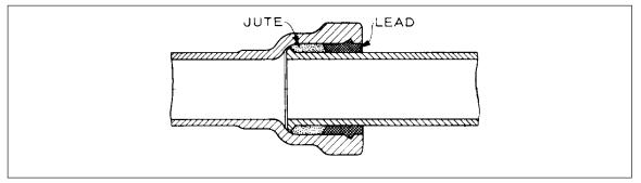
Fig. 20. Bell and spigot lead joint.
