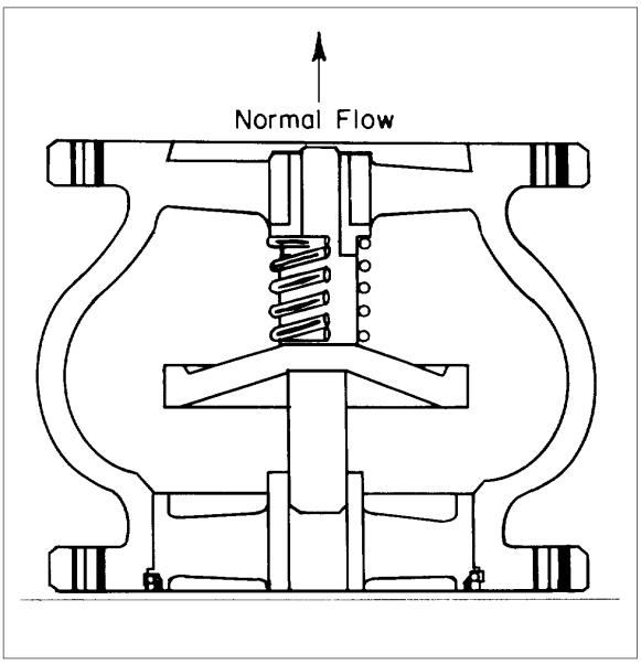
Fig. 7. Anti-water hammer check valve.
