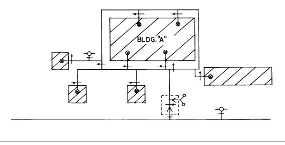
Fig. 33. System with looped main substituted for manifolded riser arrangement of Figure 32.
