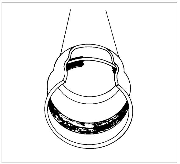
Fig. 25. PVC pipe end with integral bell and steel-band-reinforced elastomeric gasket.
