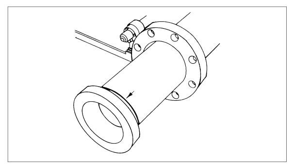
Fig. 24. Stub end butt fused to polyethylene pipe. Note joining point.
