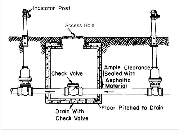
Fig. 6. Single check valve in concrete pit.
