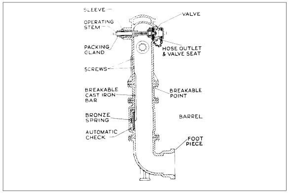
Fig. 17. Wet barrel hydrant.
