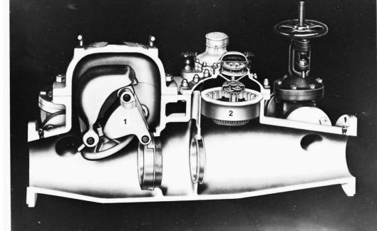
Fig. 2. Full registration fire service meter, section view showing weighted lever valve (1) and mainline torrent meter (2).
