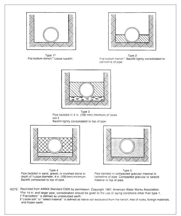
Fig. 35. Laying conditions for ductile-iron pipe.
