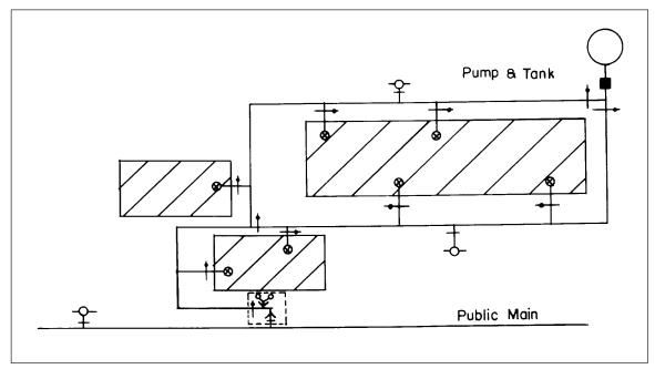
Fig. 31. Acceptable arrangement of multiple water sources.
