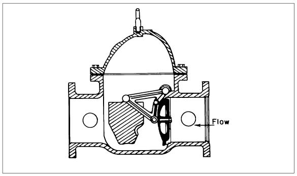
Fig. 3. Waterflow detector check valve, section view showing weighted clapper arrangement.
