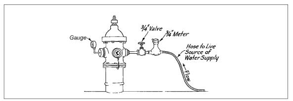
Fig. 43. Metering method of leak detection.
