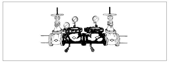
Fig. 8. Double check valve.
