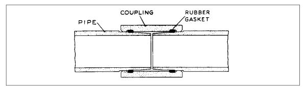
Fig. 21. Coupling for asbestos cement pipe.
