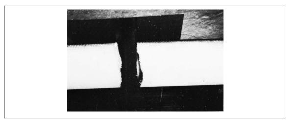
Fig. 42. Flex failure. Break offset to show crack.
