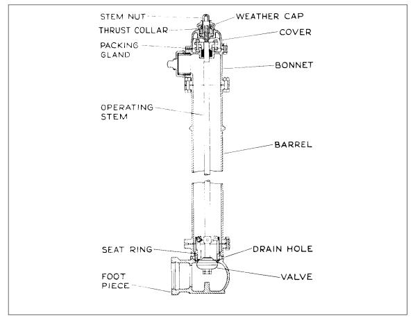
Fig. 16. Dry barrel hydrant.
