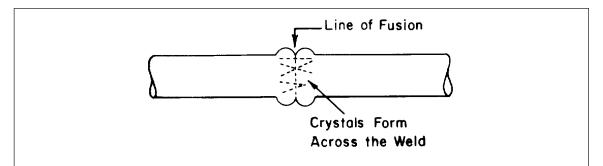
Fig. 22. Butt fusion joint.
