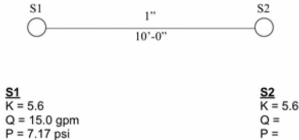
Sprinkler S1 has a K-factor of 5.6, is flowing 15 gpm, and requires a pressure of 7.17 psi. The friction loss per foot is .075 psi. As a result, .75 psi is needed for friction loss to move the 15 gpm from sprinkler S2 to S1. Therefore the total pressure at sprinkler S2 is 7.92 psi (7.17 + .75). By utilizing the formula  $Q = K \sqrt{P}$  we can solve for how much water will be discharged from sprinkler S2.
