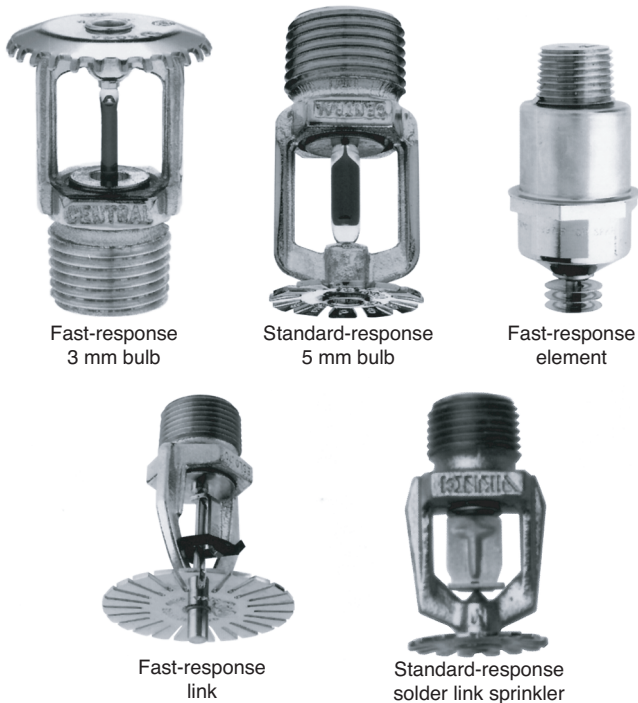
FIGURE A.5.3.1.1.1 Sprinkler Operating Element Identification.
