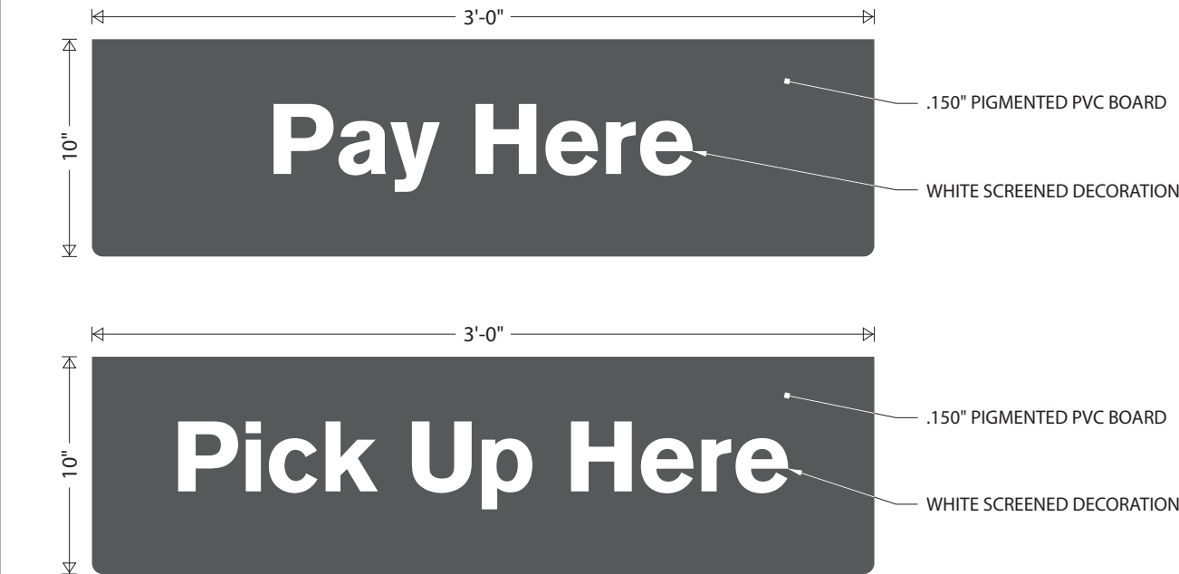
WINDOW POSITION SIGN DETAILS SCALE: 1 1/2" = 1'-0"
