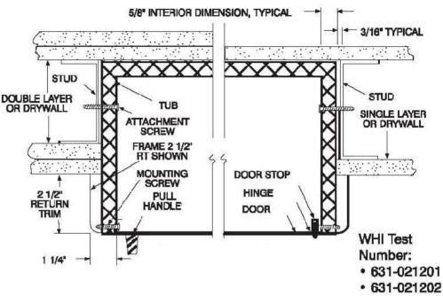
NOTE: The installation of any fire-rated cabinet which lacks a cabinet door, or any condition in which the door is left ajar, will void the fire rating
