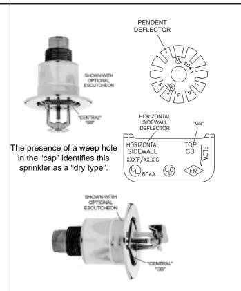
Figure 52 GB, K=5.6, Dry Pendent & Hor. Sidewall CENTRAL
