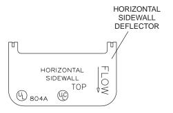
Figure 56 ELOC, K=5.6, Dry Horizontal CENTRAL
