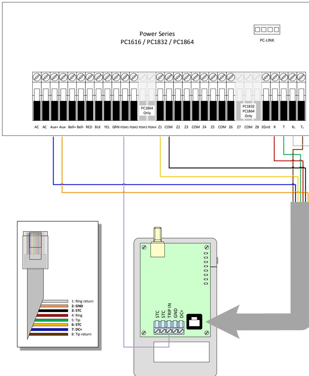
**Note:** Although a resistor is not depicted here, one may be required by the Keyswitch zone in accordance to the Panel's specifications. For more information, please refer to the Panel's Installation and/or Programming Manuals.
