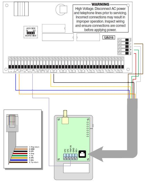
**Note:** Although a resistor is not depicted here, one may be required by the Keyswitch zone in accordance to the Panel's specifications. For more information, please refer to the Panel's Installation and/or Programming Manuals.
