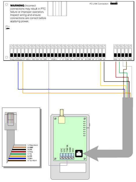
**Note:** Although a resistor is not depicted here, one may be required by the Keyswitch zone in accordance to the Panel's specifications. For more information, please refer to the Panel's Installation and/or Programming Manuals.
