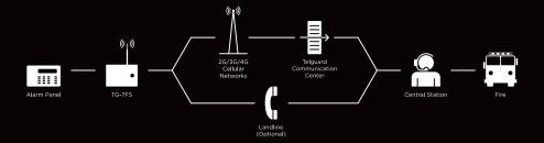
Telguard technology allows full data reporting for unlimited point-to-point signal details and maximum transmitting power for superior in-building penetration.
