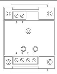
The Signature Series Single Input Module (model CT1) is an analog addressable device used to connect a Class B, normally open, alarm, supervisory, or monitor type dry contact initiating device circuit (IDC) to a Signature loop controller. One device address is required. See Table 1 for a list of model numbers.
