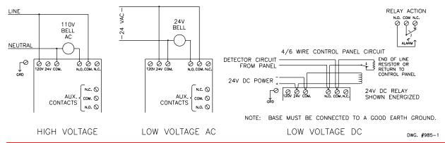
Fig. 3 Switch Terminal Connections Clamping Plate Terminal
