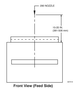
DUKE Chain Broiler With or Without Catalyst View Exhaust Deflector Size – 6.25 in. (159 mm) x 26.75 in. (679 mm):
