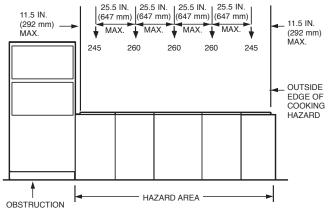
**Note:** On continuous appliance protection, start and end with 245 nozzles and 260 nozzle(s) in the middle.
