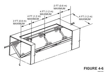
When protecting plenums with the 1W nozzle, two options of coverage are available:
