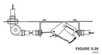
▶ 10. Insert cocking lever (Part No. 441042 or Part No. 441041) on left side of the release mechanism, with the movable flange resting securely against the corner of the cartridge receiver and spring housing, and with the notched lever portion engaging the cocking pin on **both** sides of the release mechanism. See Figure 5-32.
