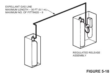
4. If an actuation gas line is connected to the regulated release assembly along with an expellant gas line, the total combined length of the gas lines **must not** exceed 30 ft (9.1 m) when using a "double-tank" nitrogen cartridge or a 101-30 CO<sub>2</sub> cartridge. See Figure 5-17.
