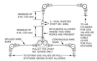
TWO WIRE ROPES CONNECTED BETWEEN A PULLEY ELBOW AND A PULLEY TEE
