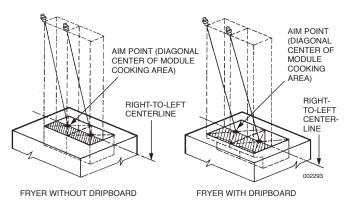
THE 3N NOZZLE TIP MUST BE POSITIONED ANYWHERE ALONG OR WITHIN THE PERIMETER AND FORWARD OF THE RIGHT-TO-LEFT CENTERLINE OF THE COOKING AREA. THE AIMING POINT OF THE NOZZLE MUST BE AT THE DIAGONAL CENTER OF THE MODULAR COOKING AREA.
