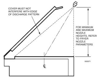
FRYER NOZZLE USED FOR TILT SKILLET OR BRAISING PAN PROTECTION MUST BE POSITIONED NEAR THE FRONT EDGE OF THE PAN AND AIMED AT THE FRONT TO BACK CENTERLINE OF THE PAN. THE DISCHARGE FROM THE NOZZLE(S) MUST COMPLETELY CLEAR THE PAN COVER WITH AN UNOBSTRUCTED VIEW TO THE BACK OF THE PAN.
