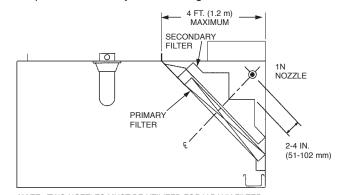
NOTE: TWO NOZZLES MUST BE UTILIZED FOR V-BANK FILTER
