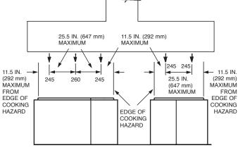
GROUP APPLIANCE PROTECTION Note: On group appliance protection, start and end of EACH zone group must be protected with a 245 nozzle.
