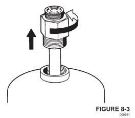
11. Make certain that each tank is filled with 1.5 (5.8 L) or 3.0 (11.6 L) gallons of only ANSULEX Low pH Liquid Fire Suppressant. Fill level to be ONLY to the level indicated in the "Installation" section. See Page 5-3, Figure 5-6, for detailed filling tolerances.
