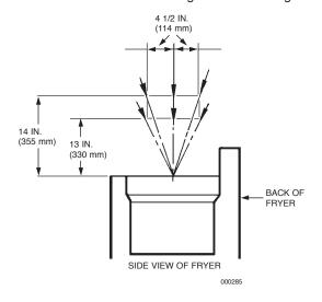
290 NOZZLE LOCATED ON FRONT-TO-REAR CENTERLINE  $\pm$  4.5 IN. (114 mm) FROM SIDE TO SIDE CENTERLINE AND AIMED AT CENTER OF COOKING AREA.
