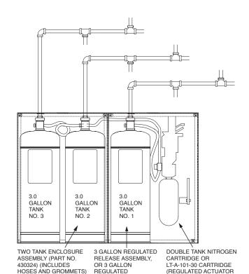
NOTE: WHEN THREE 3.0 GALLON TANKS ARE CONNECTED TO ONE AUTOMAN REGULATED RELEASE ASSEMBLY, NO ADDITIONAL REGULATED ACTUATOR(S) ASSEMBLIES CAN BE USED.
