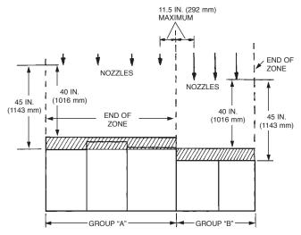
Note: On group appliance protection, start and end of EACH zone group must be protected with a 245 nozzle.
