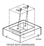
290 NOZZLE TIP POSITIONED OVER THE MIDPOINT OF THE RESPECTIVE MODULAR
