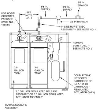
NOTE 1: THE PIPE CONNECTION FROM TANK CENTER TO TANK CENTER CANNOT EXCEED 8 1/2 IN. (215 mm). ALSO, OEM RELEASE/BRACKET ASSEMBLY CAN BE UTILIZED WHEN MANIFOLDING 3.0 GALLON TANK.
