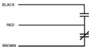
Figure 4-23. Wiring Diagram For Model MS-SPDT Micro Switch.
