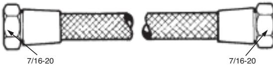
Figure 2-22. Stainless Steel Actuation Hose.
