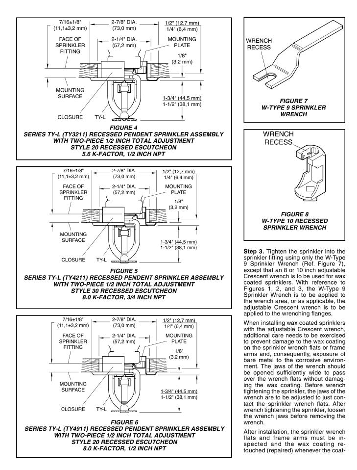
ing has been damaged and bare metal is exposed. The wax coating on the wrench flats can be retouched by gently applying a heated 1/8 inch diameter steel rod to the areas of wax that have been damaged, to smooth it back over areas where bare metal is exposed.
