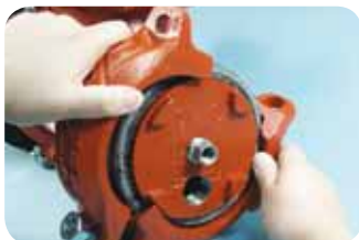
Remove coupling and closure cap
